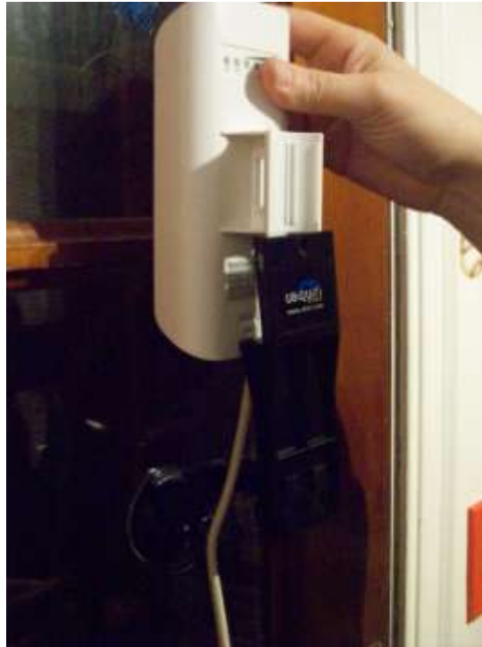
Figure 10 – Slide device onto bracket.
