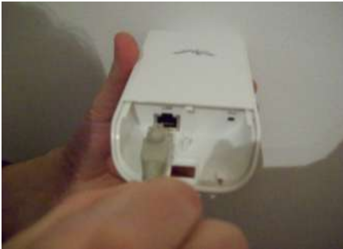
Figure 8 – Plug in cable into “LAN”.
