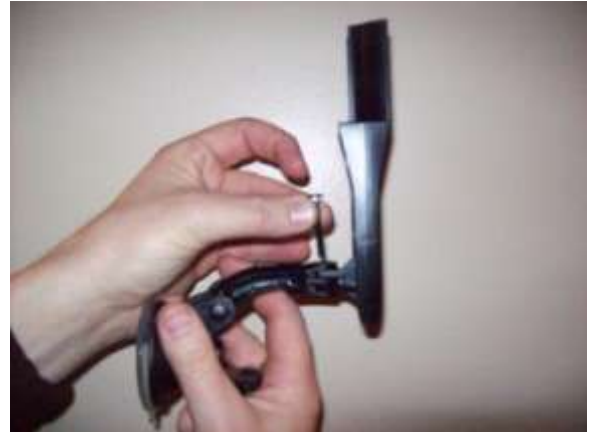
Figure 2 – Place screw into bracket arm.
